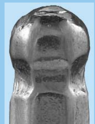
Competitor poorly machined
